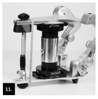
Fixate the articulator closed with the aid of a rubber band and allow the adhesive to cure.
