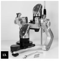
Check the bond with the centring key. Loosen and remove the central Allen screw of the centring key. Pull the key apart evenly and remove the locating pins by hand. Insert the individual parts of the key into the articulator (TOP points to the upper part of the articulator).
