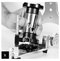
Check centring key for cleanliness of mating surfaces, check Allen screw & tighten if necessary. Turn articulator upside down, place centring key on the base plate in the upper part of the articulator. The side marked "TOP" faces the base plate, the Allen screw faces the anterior tooth guide pin.
