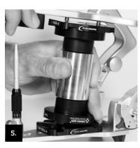
Close articulator. To do this, it is necessary to tilt the centring key slightly to the back!
