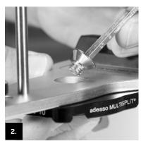
Insert the base plate in the upper part of the articulator, tighten the screw. The base plate must be mounted without gaps or play.
