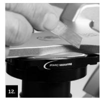
After 10 minutes, excess adhesive can be trimmed with a cutter knife. The centring key can be removed for adjusting further articulators after 60 minutes. After 24 hours, the adjustment adhesive has reached its final hardness.
