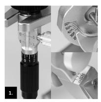
Check the articulator for possible defects. The upper part must not exhibit any play in the centric. Close the centric lock. Set the condylar inclination to 35°. The Bennet angle to 0°. The incisal pin to 0.
