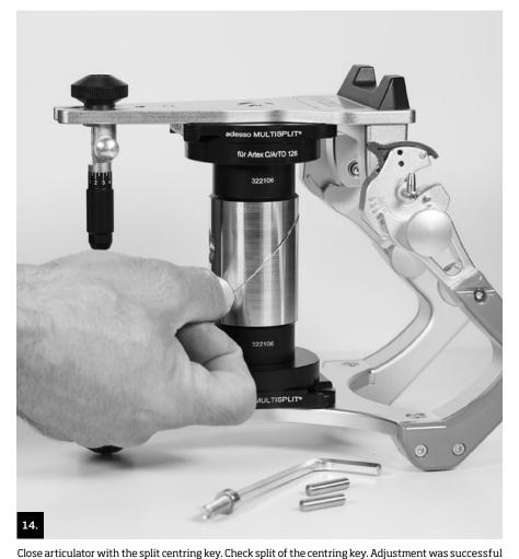
if you neither see a light gap between the split or do not feel a ridge when you run your fingernail over the split. Otherwise, synchronisation must be repeated. The locating pins should always be wetted with fine machine oil before assembling the centring key.
