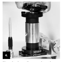
Place the clean adjustment base plate on the centring key.
