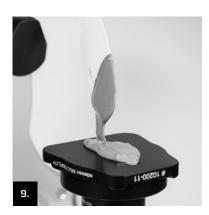
Turn the articulator upside down, open it and carefully apply the adjustment adhesive to the adjustment base plate. It is essential to fill the drill holes with adhesive.
