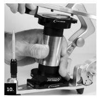
Carefully close the articulator. To do this, it is again necessary to tilt the centring key slightly to the back!
